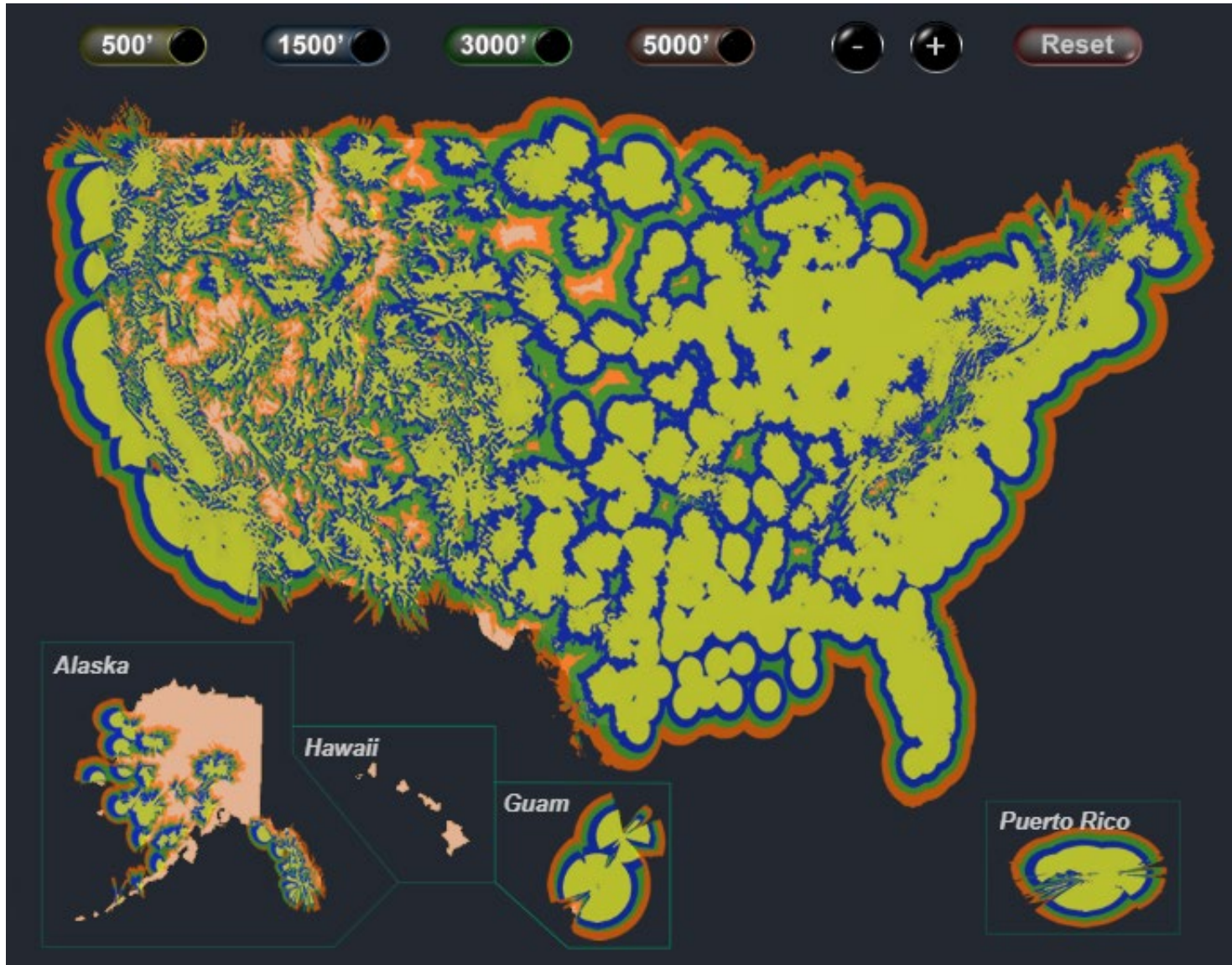
Figure 2. Automated Dependent Surveillance-Broadcast Ground Stations Coverage Map (including the location of 600 ground stations)
