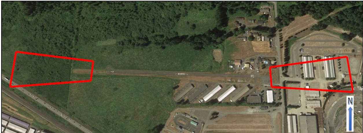
Figure 2-60. First Air Field Runway Protection Zones
