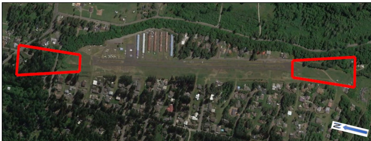
Figure 2-40. Norman Grier Field Runway Protection Zones
