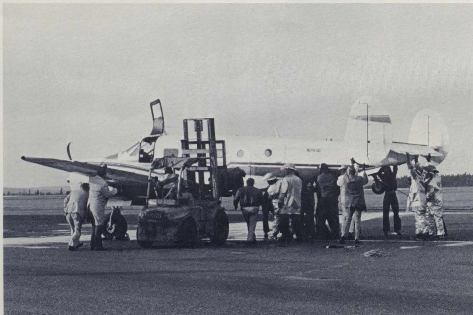
Men and forklift carefully brought down the plane to a position parallel with the ground, and the forklift was removed.
