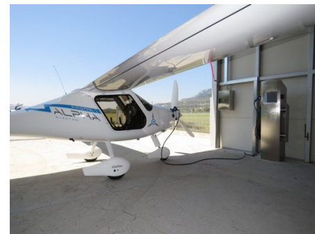
Pipistrel electric aircraft charging station. Source: SustainableSkies.org
