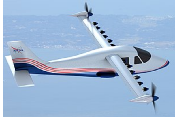
The NASA X-57 "Maxwell" is the agency's first all-electric aircraft and is used to validate and demonstrate the benefits of distributed electric propulsion. Source: NASA
