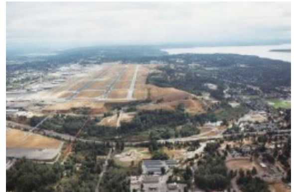
Sea-Tac Airport August 2003 from the north The runway to the west is the new taxiway. Mounds of earth to the west of the taxiway are third-runway fill.
