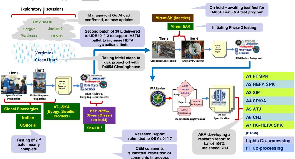
\*Fuels approved via ASTM D4054 and annexed under D7566 are considered **synthetic blend components** (SBC). Current annexes require that SBCs be blended with conventional jet fuel. Once blended, the fuel meets ASTM D1655 criteria for aviation turbine fuel.
