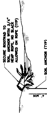
DETAIL 4 NO SCALE TYPICAL HABITAT LOGS (TYPICAL)
