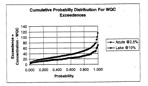
The probability that the WQC annual exceedence for total dissolved copper was greater than 40 ug/L for an event with a probability of approximately 67 percent (once in three years). This is seen in the following figure. The results are somewhat sensitive to the lake criterion for allowable mixing volume. In comparison, the WQC exceedence for total dissolved copper was greater than 25 ug/L approximately 67 percent of the time.
