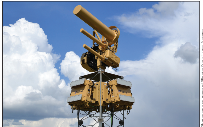
The Anti-UAV Defence System (AUDS) uses electronic scanning radar to detect drones up to 6 miles away and radio waves to disable them
