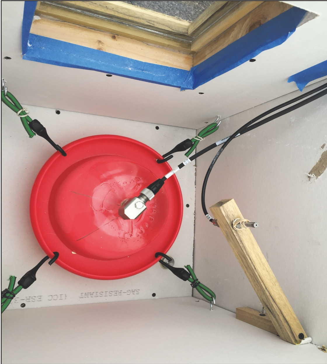
Figure 13. Instrumentation setup for the microphone and accelerometer.
