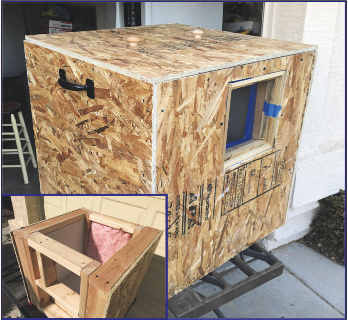
Figure 12. Structural mock-up platform for data collection.
