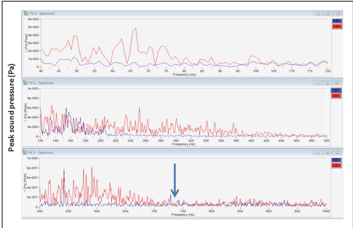
Figure 16. Open-air attenuation frequency for sound energy. Each graph continues the frequency of the previous. The smallest amplitude pressure on each y-axis from the previous frequency was used to set the starting point frequency for the next figure. This was done to magnify the data for improved inspection.
