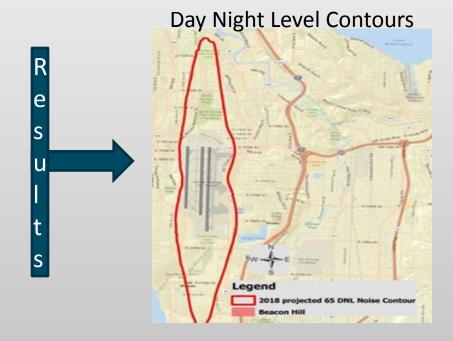
DNL is a cumulative metric required by the FAA – 65 DNL is the area the FAA allows for mitigation
