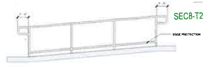
2 ADA HANDRAIL DETAIL 1/2" = 1'-0"
