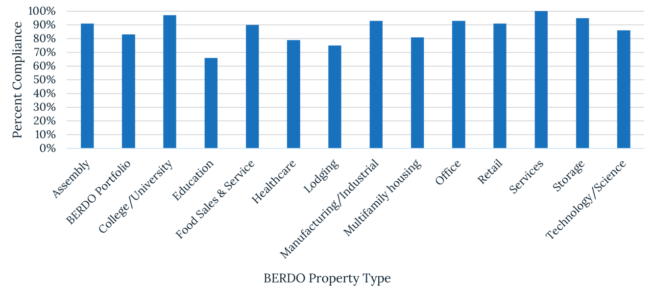
Figure 9: Based on 2024 BERDO-reported data, the City projects that approximately 84 percent of BERDO-covered buildings will meet their 2025 emissions limits. This projection assumes no participation in BCCE or renewable energy credit (REC) purchases, which buildings can use to reduce their reported emissions.
