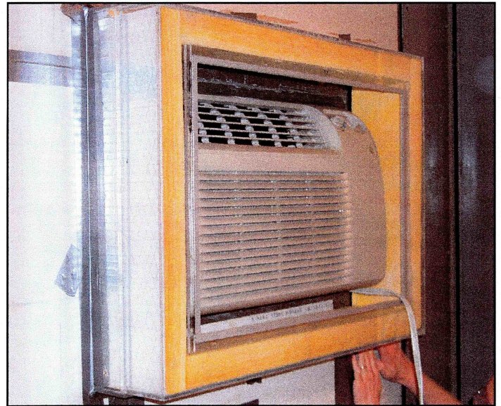
Acoustical Test Setup for Pull-Through Air Conditioners
