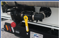
GLYCOL RECOVERY FOR PICKING UP DE-ICING FLUID
