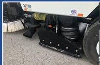
VACUUM AND BRUSH REMOVAL OF DEBRIS
